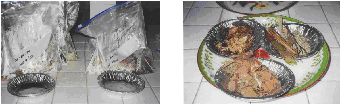
FIGURE 2-14: MOISTURE CONTENT SAMPLES COLLECTED IN ZIPLOC BAGS (LEFT) BROWN ORGANICS IN ALUMINUM DISH (RIGHT)
