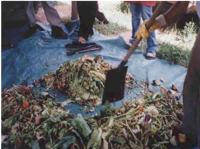
FIGURE 2-13: CONING AND QUARTERING TECHNIQUE
